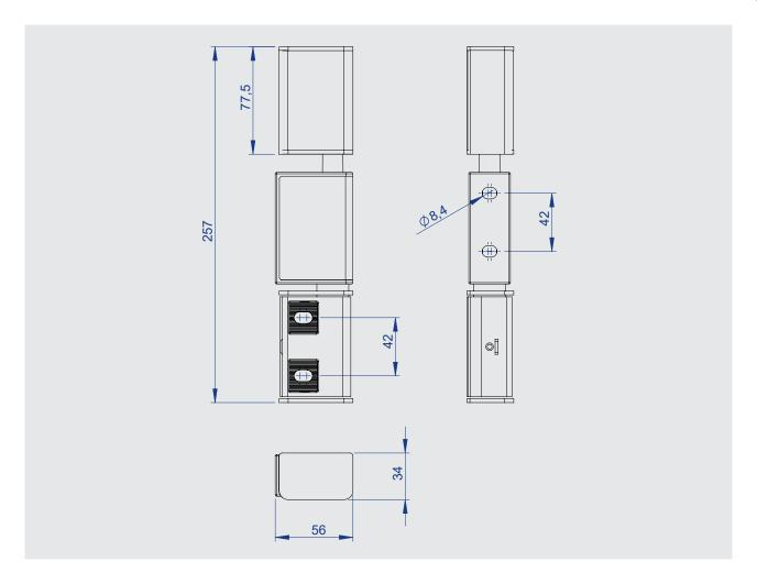
This edge-mounted hinge offers perfect closure with plastic. It may not look like it in view of its stainless steel appearance, but it really is plastic. The extremely robust hinge is corrosion-resistant, rising and has a load capacity of up to 80 kg in the double pack — seriously impressive. At the same time, it can be adjusted in three axes and is available as right and left version. This hinge simply offers more than you would think.
