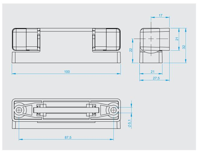
Closing? No problem! With its optional spring, this hinge offers a very special experience when it comes to closing. With an opening angle of less than 45°, the door closes almost by itself. Another nice thing: You don't have to exclude security with this hinge. Its caps act as dismantling protection, because they can only be slid on and off when the door is open. The load capacity of two edge-mounted hinges is about 20 kg. The maximum opening angle is 190°.
